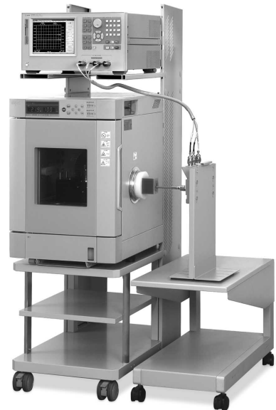
Figure 22. The E4991A Option 007 with the ESPEC bench-top temperature chamber (SU-261)
